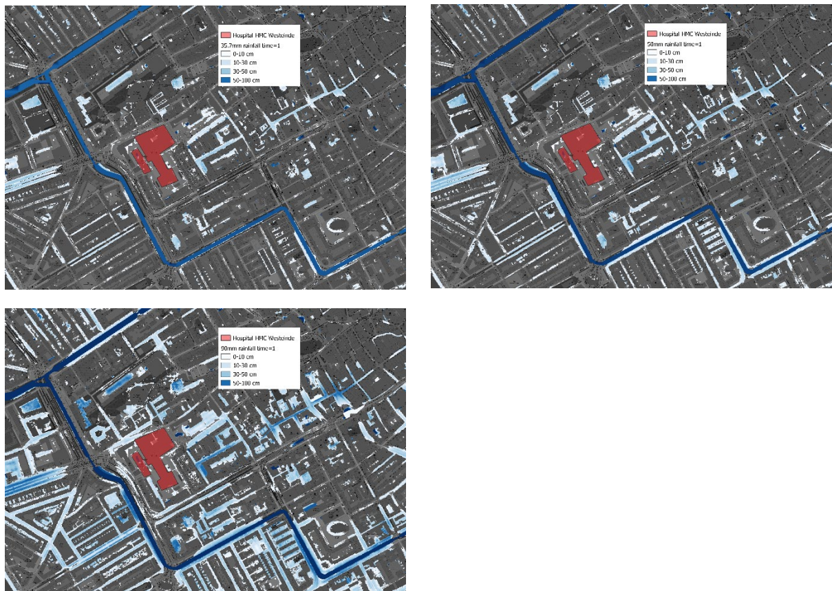
Figure 38 a, b, c: Details of the inundation maps of the area around HMC Westeinde for a rainfall of 35.7mm (a) 50mm (b) and 90mm (c).
