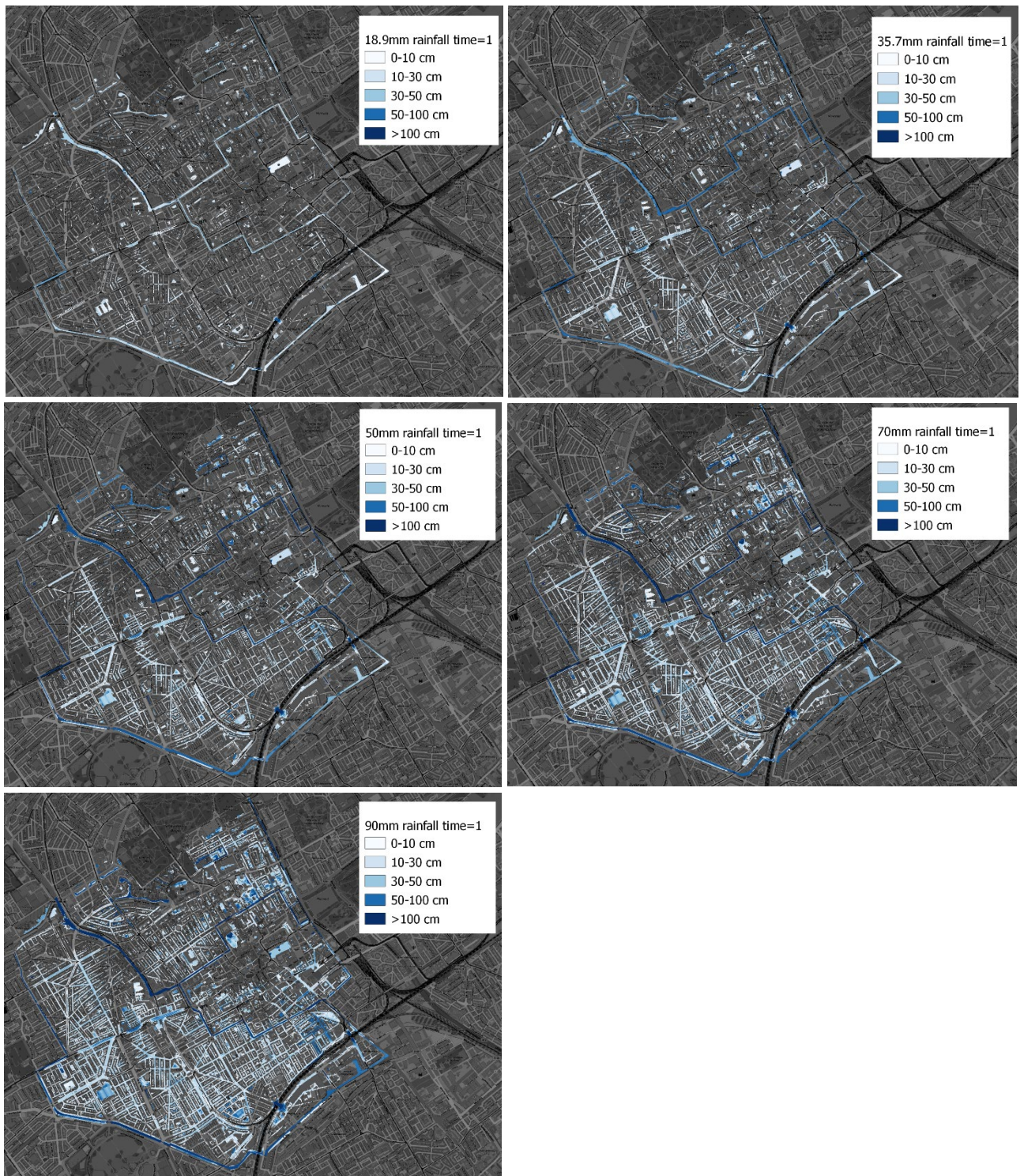
Figure 29a, b, c, d, e: Inundation maps retrieved from 3Di of 5 different rainfalls at the point in time directly after the rain event (time=1).
