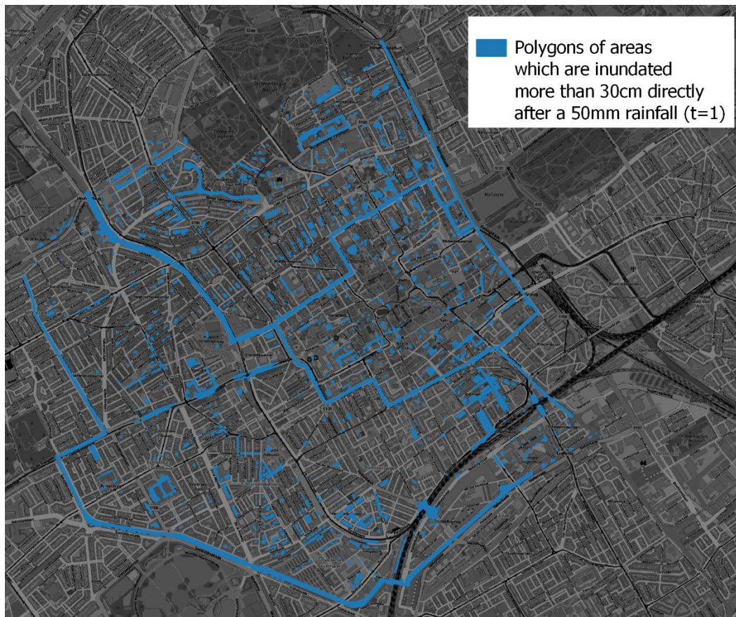
Figure 23: An example of the polygons representing inundated areas of over 30cm.
