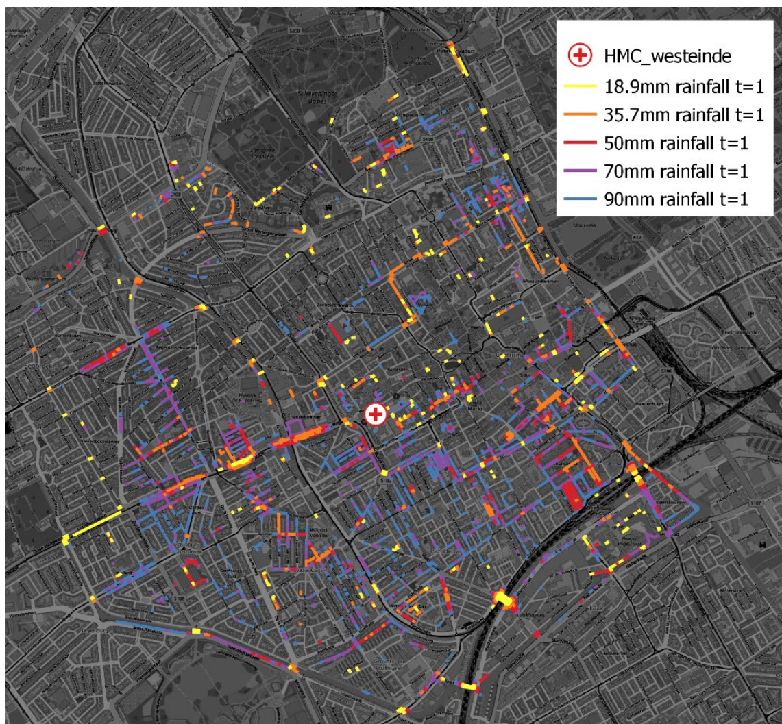
Figure 32: Road segments inundated at least 30 cm directly after the rainfall (t=1). Different colours indicate the different rainfalls simulated in 3Di.
