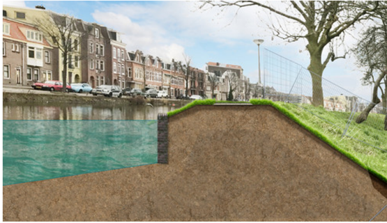
Figure 2.7: Hybrid flood protection (De Ingenieur, 2020)
