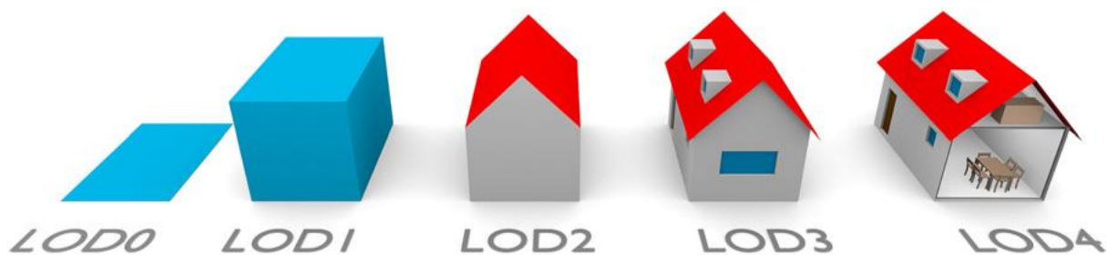
Figure 19 The level of detail in CityGML 2.0 (Biljecki, Ledoux, & Stoter, 2016).
