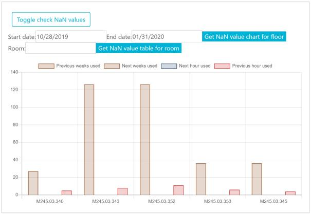
Figure 59: NaN values found for comfort data on the third floor
