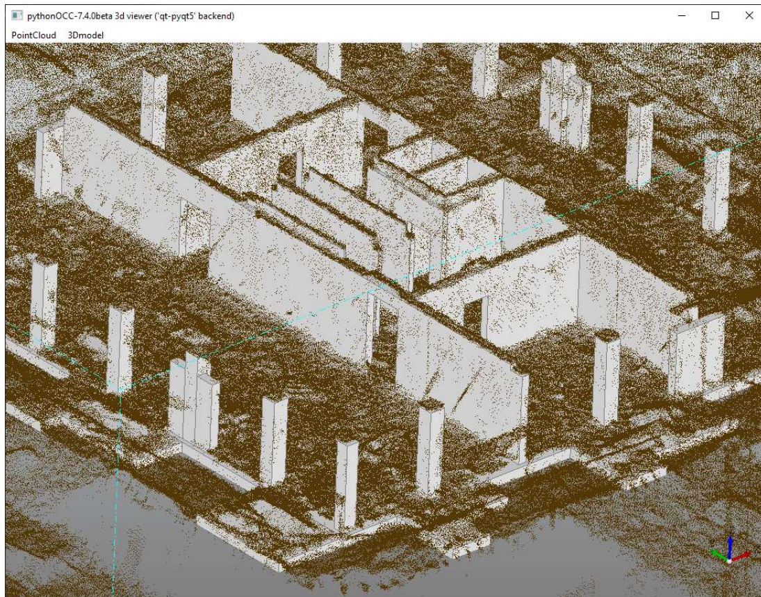
Figure 43: The point cloud data with the 3D model together
