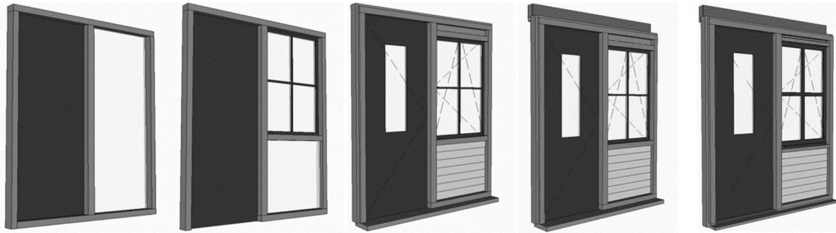
Figure 31: LOD 100 - LOD 400 of a door (Hermans, 2015)
