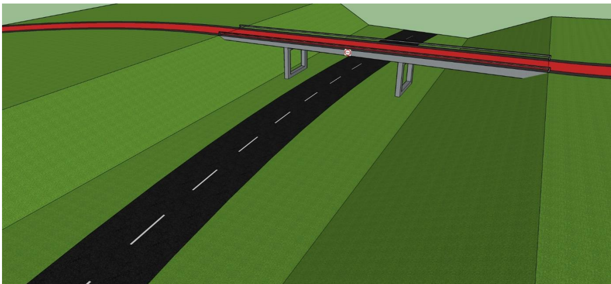
Figure 10. Visualization of multiple IFC objects with a 3D engine: A road and a bridge
