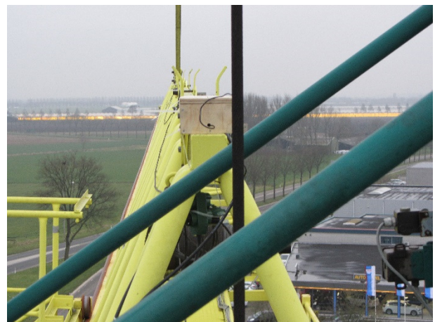
Figure 51. Sensor placed on top of the crane's jib
