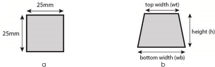
Figure 22: a) Nozzle dimensions, b) Printed layer cross section
