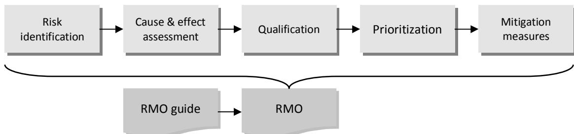
Figure 2.2: The position of the tools/documents in the current RM method structure
