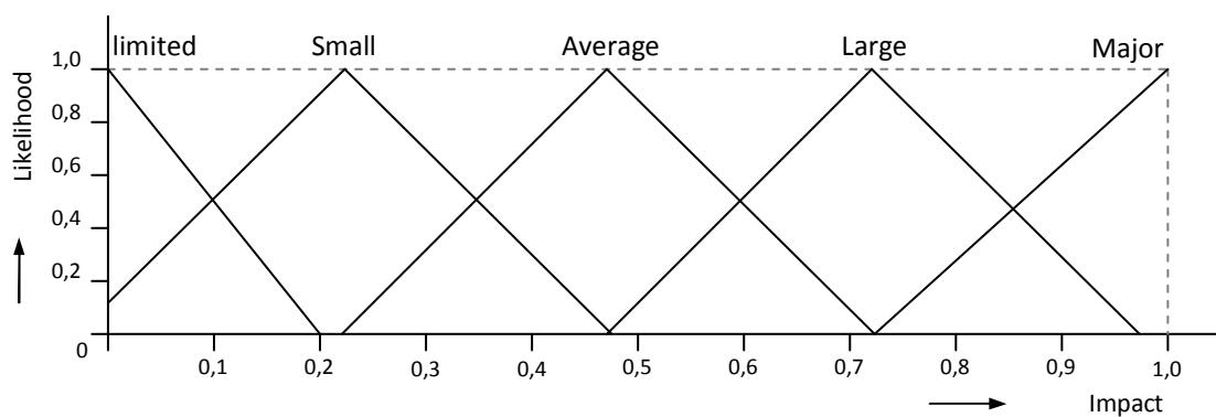
Figure 5.5: Visualization of the membership functions of the TFN's in the factor Quality
