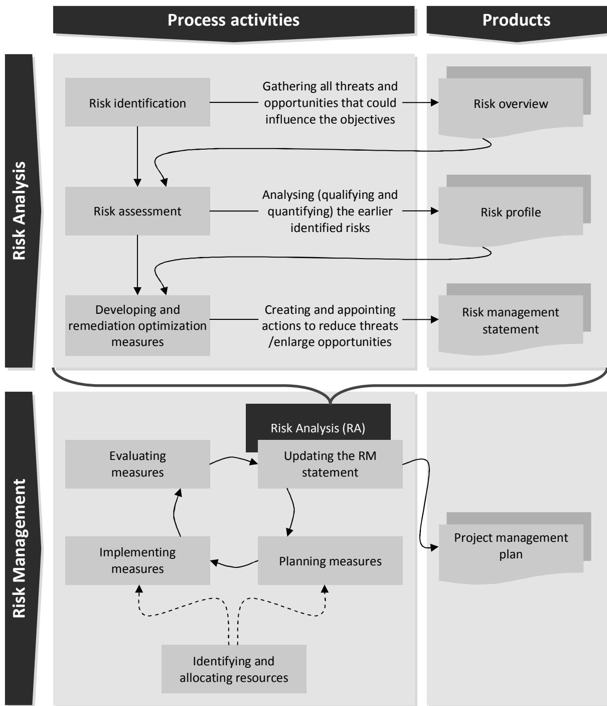
Figure 4.2: Proposed RM framework including the selected activities and products embedded in their respective RM principle; the framework focuses on the internal process, hence the overarching strategic step is, currently, omitted.
