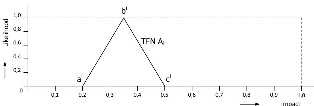
Figure 5.4: visualization of the TFN A and its distribution based on the experts values.
